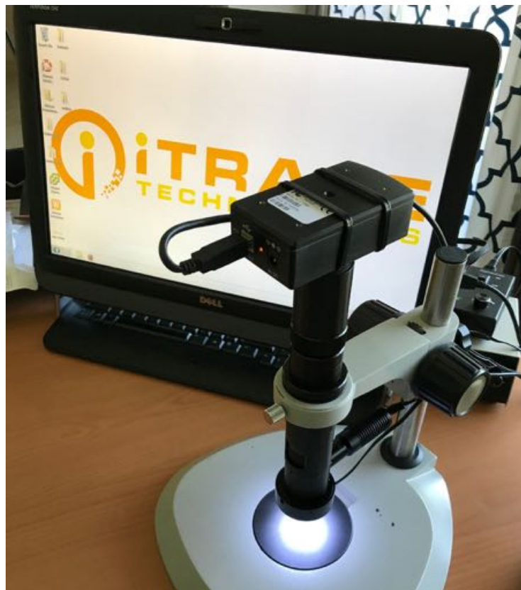
iTRACE micro mark inspection station with Lumenera Lu105 camera and 75X optics
